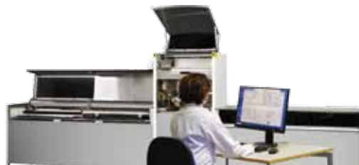
Itrax Core Scanner samples are inserted in the left wing, and automatically moved during scanning. The user sets the scan parameters from the computer, and can then leave the instrument to apply the measurements unattended.
