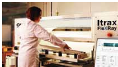
The pull-out sample holder makes it convenient, quick and safe to switch samples, whether these are sediments in liners or drill cores.
